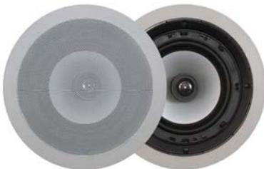
The EMOtion 6 RO are premium two-way systems with very rigid 6,5" aluminium cone woofers and high-power 0,75" ferrofluid cooled aluminium dome tweeters. These speakers combine precise dry bass with incredible openness in the midrange and crystal-clear highs. They excel by bringing every musical detail to life and by the precise spatial positioning in both low and high volume situations. Power and accuracy at an incredible price, but no compromise to quality.
